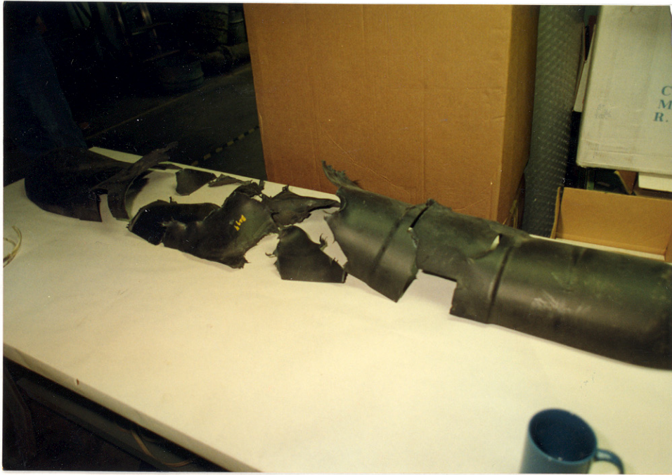
25. Shattered HDPE Shield from the Ruptured Cylinder
